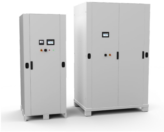
Figure 5: REGATRON's liquid-cooled system solutions up to IP54 with various power levels e.g. 54...162 kW (left) and 216...324 kW (right). The remote control unit RCU, indicator lights, emergency stop button, and main switch allow the user to operate the system on the enclosure's front door.
