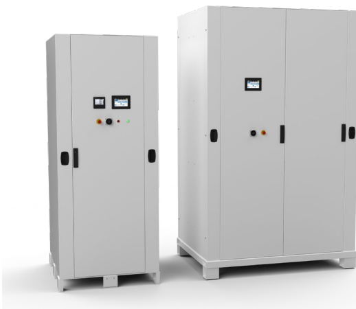
Figure 5: REGATRON's liquid-cooled system solutions up to IP54 with various power levels e.g. 54...162 kW (left) and 216...324 kW (right). The remote control unit RCU, indicator lights, emergency stop button, and main switch allow the user to operate the system on the enclosure's front door.
